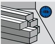
Allow the panels or tiles to acclimatize in the relevant room for at least 48 hours, lying flat, at a
